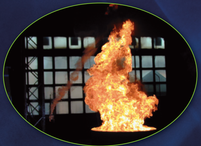
A controlled heptane pool fire conducted for the purpose of fire model validation. Courtesy Simo Hostikka, VTT Research Centre, Helsinki, Finland
