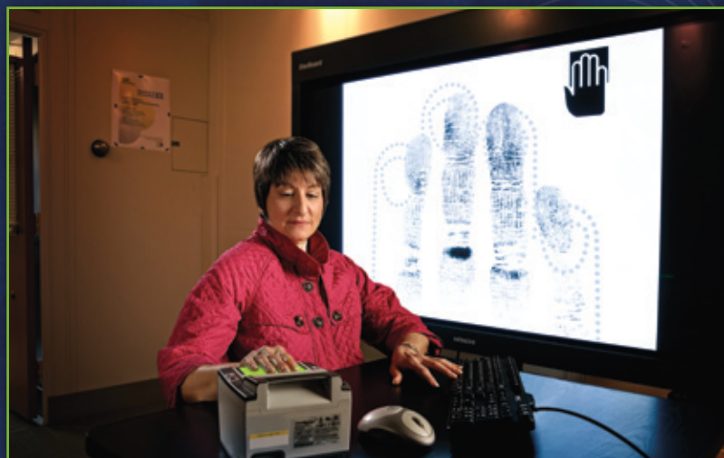
Computer scientist Mary Theofanos demonstrates a NIST-developed system that visually guides users to correctly place their hands on a digital fingerprint scanner. The system improves image quality and speeds up the fingerprinting process by allowing a person to provide prints unassisted.
