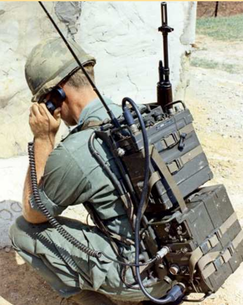
The NESTOR system was developed in answer to the military's need for lighter and more efficient communication systems. The Soldier above is using the KY-38 "manpack."
