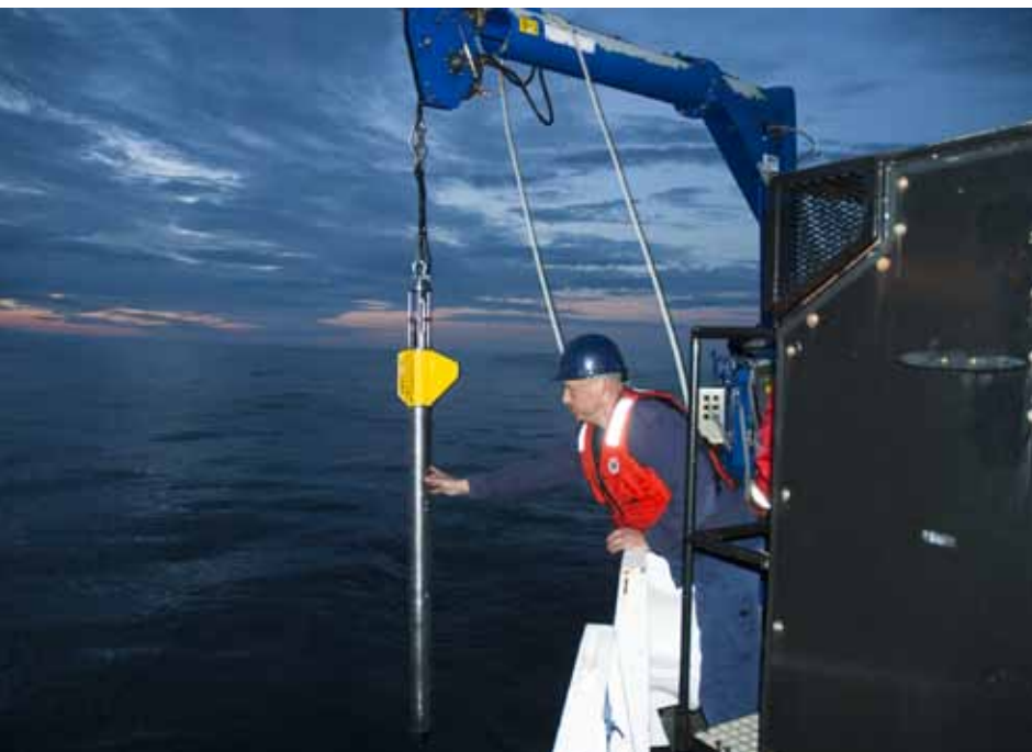
Figure 14. Free-fall cone penetrometer ready for deployment. Sensors in the body of the instrument measure deceleration as the device penetrates the seafloor and comes to rest below the surface, providing information about the vertical structure of sediments while the ship is underway. Another sensor in the yellow tail region measures sound velocities in the water column which are used to provide high-quality acoustic data.
