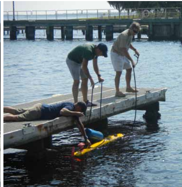
Fig. 15. NOAA personnel preparing a new HarborScan AUV for shoreside deployment at the NMFS Panama City Laboratory.
