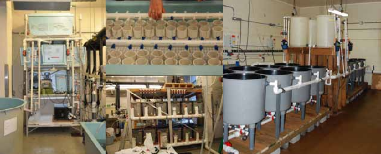
Figure 3. Experimental CO 2 dosing systems at the Kodiak and Newport Laboratories.
