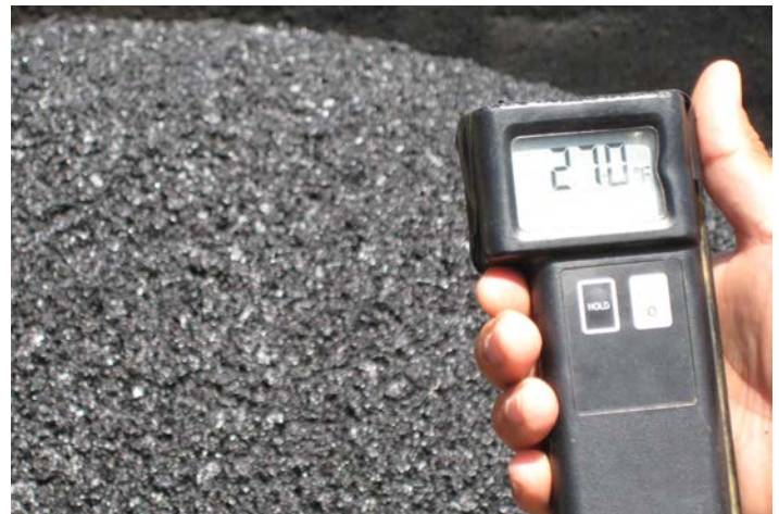
Warm mix asphalt typically requires lower temperatures which are friendlier to construction workers and to the environment
