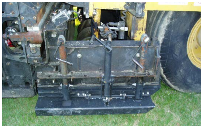
Similar devices mount on the paver's end gate
