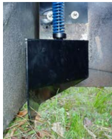
Similar devices mount to the paver's screed
