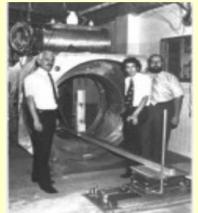
The world's first magnetic resonance scanner (1977). NSF-supported research led to the development of MRI technology. Credit: Courtesy FONAR Corporation.
