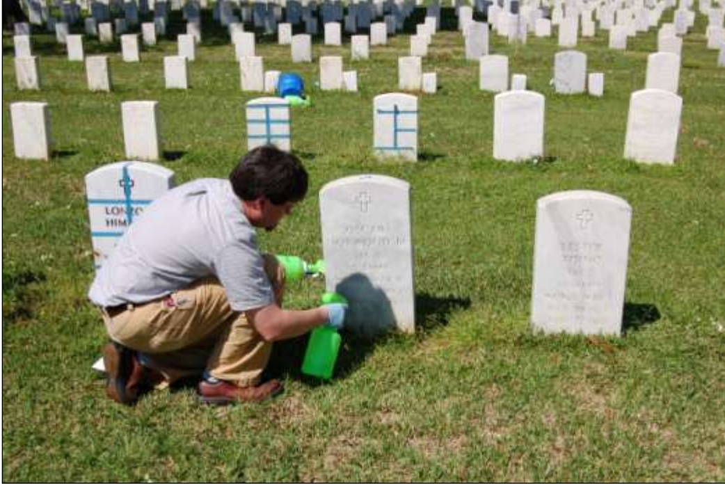
Jason Church tests cleaning solutions on headstones at Alexandria National Cemetery, Pineville, LA.
