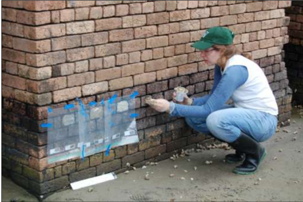
Katherine Langdon compares poultice recipes for crude oil removal at Fort Livingston, Grand Isle, LA.
