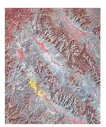
The yellow line in this Landsat satellite image indicates the rupture along the Lost River fault during the 1983 earthquake. The large yellow circle near the bottom locates the main shock Smaller circles represent aftershocks in proportion to their magnitude. The yellow square north of the fault is the town of Challis. by Ross Stein and Robert C. Bucknam
