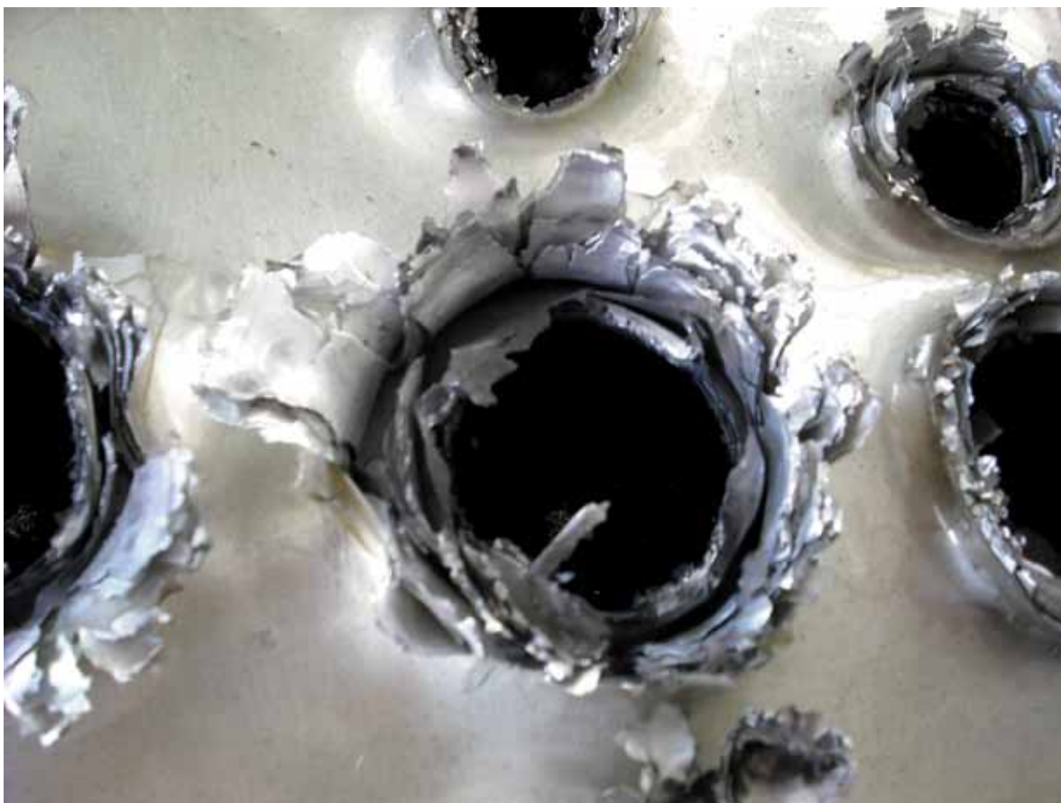
FIGURE 3 Profuse damage accompanying penetration of laminate with 21 alternating elastomer and aluminum layers.
