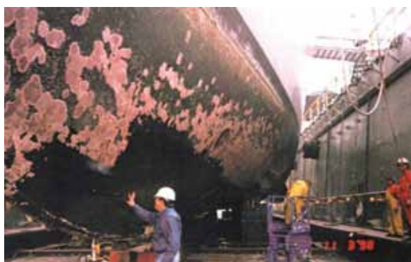
FIGURE 1 Fouling of ship hulls results in damage to surface treatments and increased drag. This ship is encrusted with bryozoans (pink patches), an invertebrate animal.
