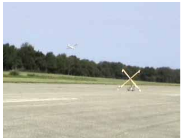
FIGURE 2 UAV in automatic approach to the simulated recovery target.
