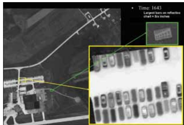
FIGURE 8 DB-WAPSS daytime MWIR flight imagery (June 9, 2009). Inset images show (top) a resolution target, and (bottom) vehicles in a magnified view of the parking area.
