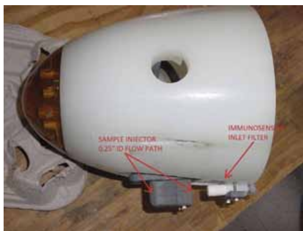
FIGURE 2 Nose of REMUS100 with plume generator and the filter capped inlet for the immunosensor.
