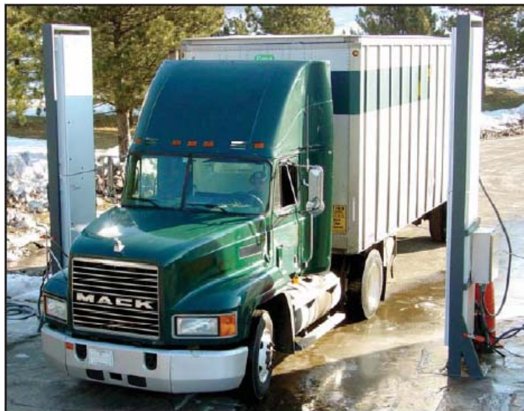
Figure D-3 Example Portal Monitor (Canberra 2005b)
