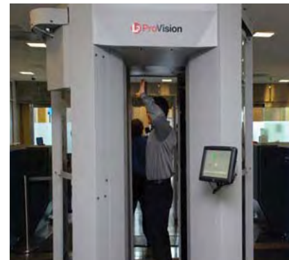
Screening of an Airport Passenger by Advanced Imaging Technology
