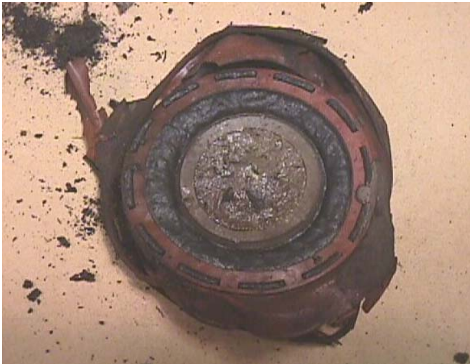
Figure 18 – Rear View of Unit #1 Regulator Diaphragm
