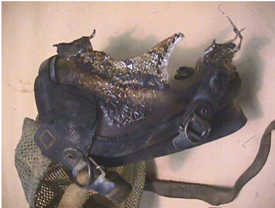
Figure 5 – Side View of Unit #1 Facepiece
