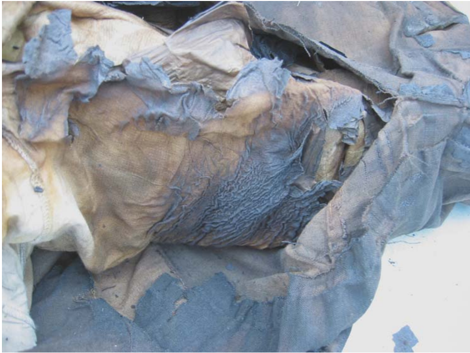
Figure 69 – Damage to Moisture Barrier of Turnout Coat
