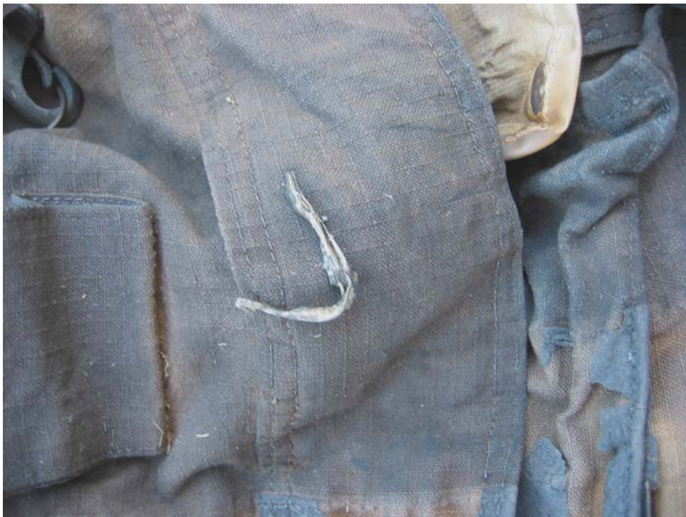
Figure 67 – Plastic Adhered to Front of Turnout Coat
