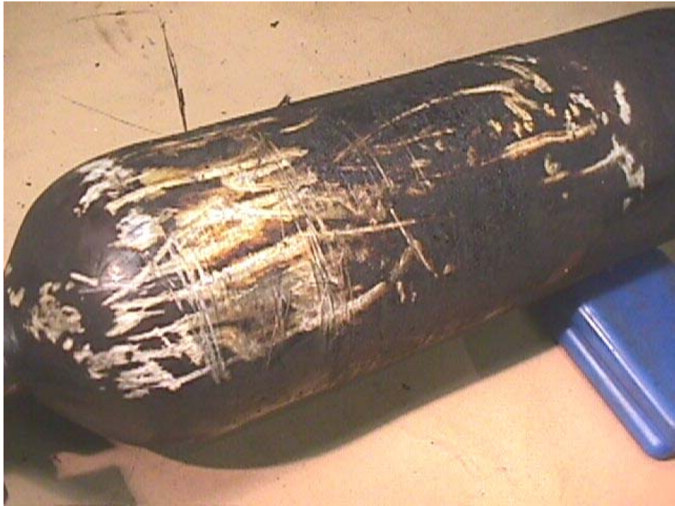
Figure 38 – Heat Damage to Unit #1 Cylinder
