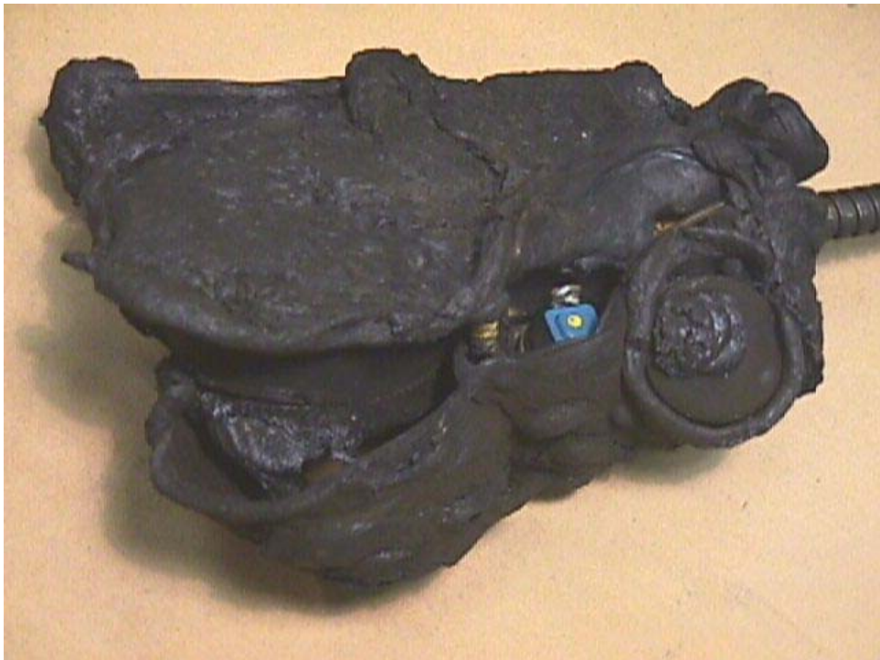
Figure 22 – Rear View of Unit #1 Remote Pressure Gauge/PASS Console
