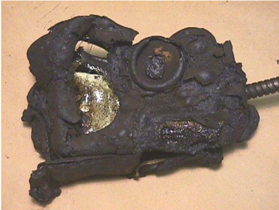
Figure 21 – Unit #1 Remote Pressure Gauge/PASS Console
