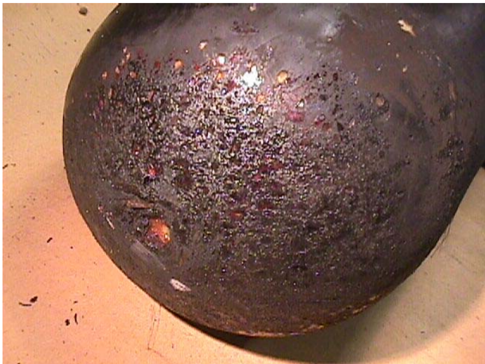
Figure 38 – Heat Damage to Unit #1 Cylinder
