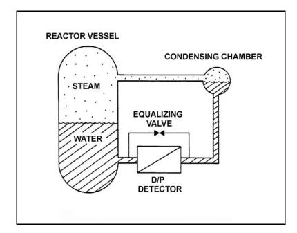
Refer to the drawing of a differential pressure (D/P) level detection system for a reactor vessel at normal operating temperature and pressure (see figure below).
