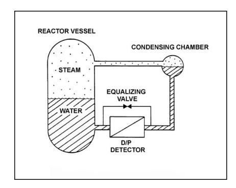
Refer to the drawing of a reactor vessel differential pressure (D/P) level detection system that was calibrated at 500 psia (see figure below).
