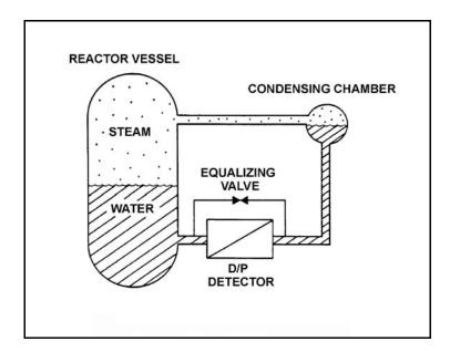
Refer to the drawing of a reactor vessel differential pressure (D/P) level detection system that was recently calibrated at normal operating conditions (see figure below). Assume that the associated reactor vessel level instrument does <u>not</u> use density compensation.
