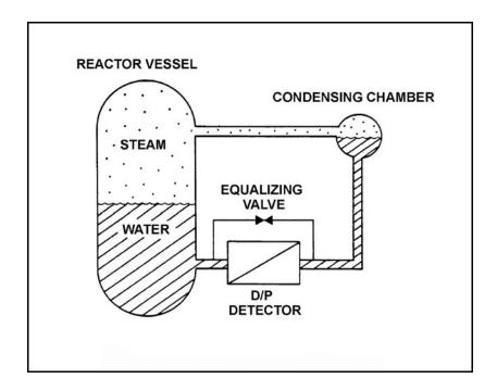
Refer to the drawing of a tank differential pressure level detector (see figure below).
