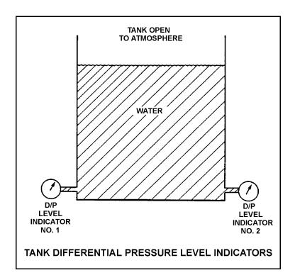
Refer to the drawing of a tank differential pressure level detector that was recently calibrated at a tank water temperature of  $80^{\circ}$ F (see figure below).
