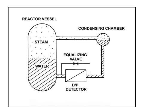
A nuclear reactor is currently shut down at 180°F. Reactor vessel (RV) level is being monitored using a normal at-power RV level instrument that was calibrated at normal plant operating conditions.
