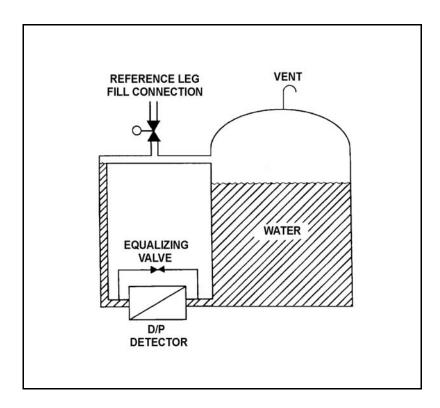
The downcomer region of a reactor vessel contains 40 feet of saturated water at 536°F. A reactor vessel water level detector has a pressure tap located at the bottom of the downcomer region. Approximately how much of the total pressure at the pressure tap is caused by the downcomer water?
