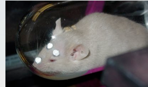
An awake mouse with infrared reflectors for head tracking shown in imaging burrow.
