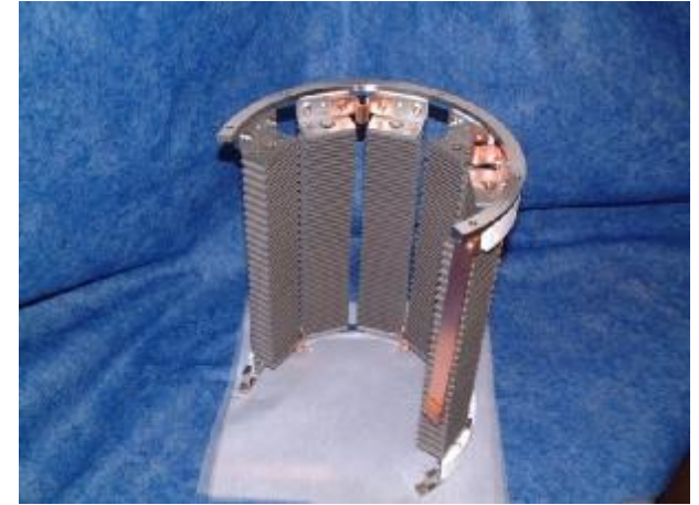
NEG pump array
