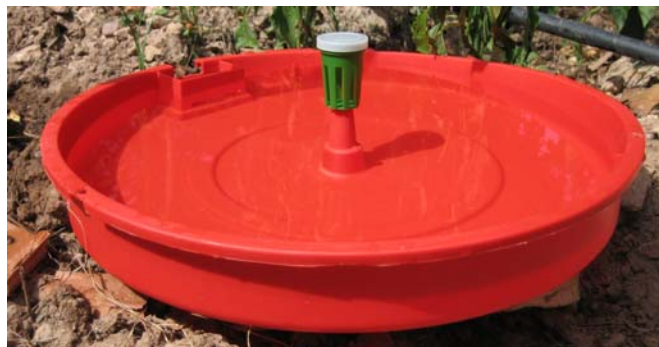
Figure 4-10 TUTASAN Pan Trap with Dripper System to Maintain Water Level (Koppert Biological Systems, http://www.koppert.com/products/monitoring/products-monitoring/detail/tutasan-watertrap-2/ )
