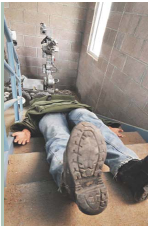
BODY RESCUE - A robot pulls a dummy of a fallen bomb technician to safety.
