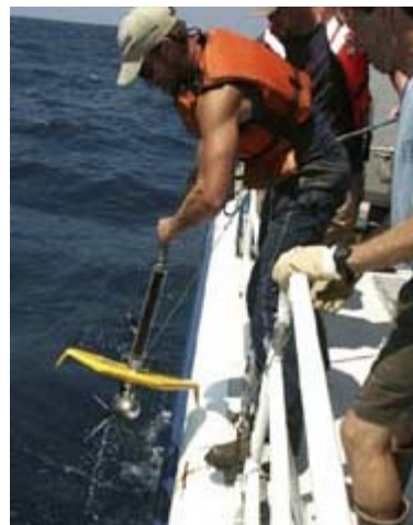
Deployment of the side scan sonar tow vehicle, also called a 'fish'. (Photo: NOAA)
