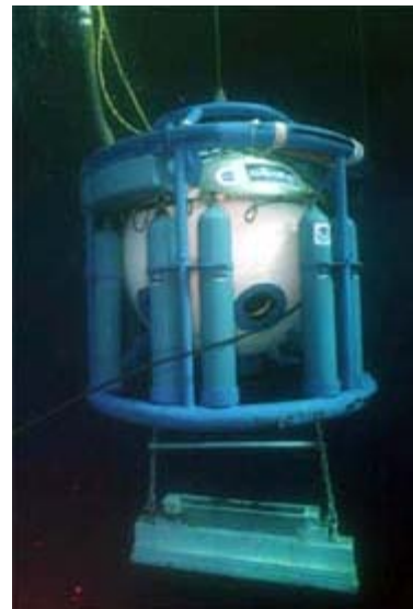
The SAT system diving bell is raised to the surface after an eight hour dive on the wreck of the USS Monitor . The bell is the divers' "taxi" between their topside saturation living quarters and their work site, some 240 ft below the surface. (Photo: official U.S. Navy photo by Photographer's Mate Chief Petty Officer (DV/SW) Andrew McKaskle)
