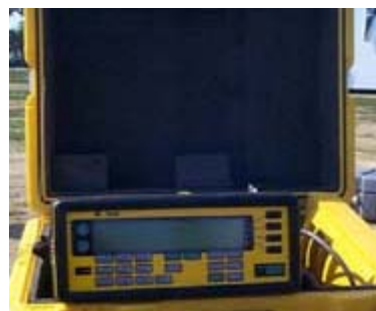
Portable GPS unit utilized in surveying.
