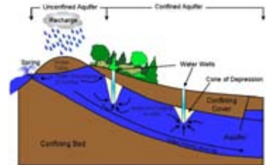
Diagram of an aquifer system. (Diagram: Texas A&M Univ.)
