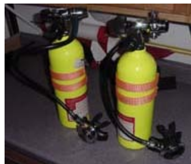
The first stage regulator is attached to the scuba tank. (Photo: NOAA/National Undersea Research Program)
