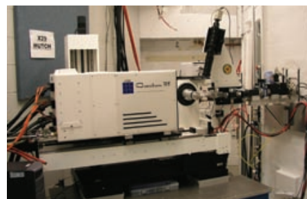
The new diffractometer and detector system in the X29 x-ray hut. This device is equipped with a high-speed and high-precision crystal axis suitable for operation with a robotic specimen changer.
