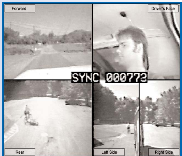
Figure 1. Split-screen presentation showing the five camera views, recording inside and outside of the heavy vehicle.
