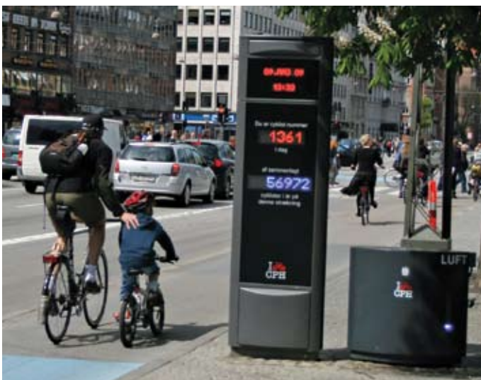
Figure 53. Bike counter (daily and year-to-date subtotals) and air pump in Copenhagen, Denmark.
