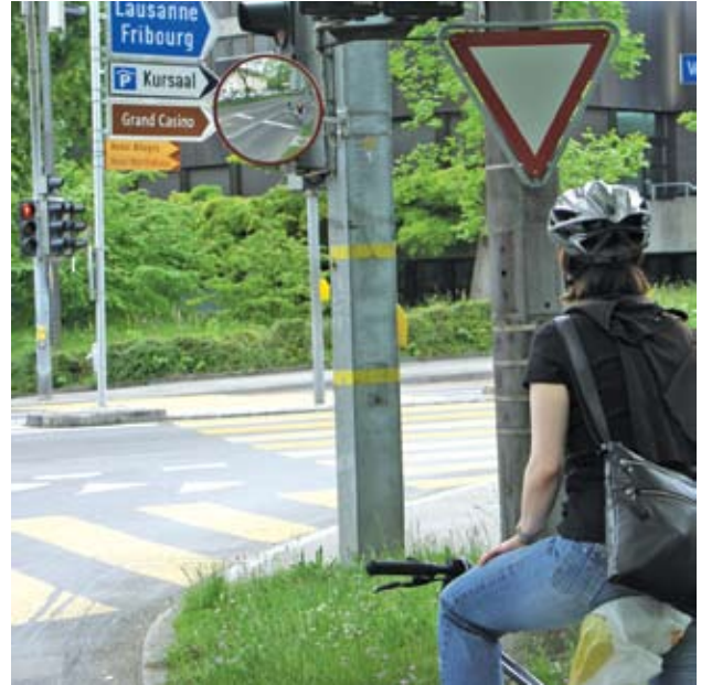
Figure 25. Convex mirrors improve bicyclist visibility for drivers of large or high-profile vehicles in Bern, Switzerland. (Note: photo taken from vantage point of motorist at stop line.)
