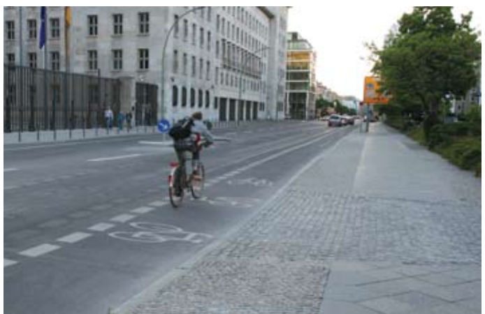
Figure 30. Bike symbols oriented to motorists turning at a driveway in Berlin, Germany.
