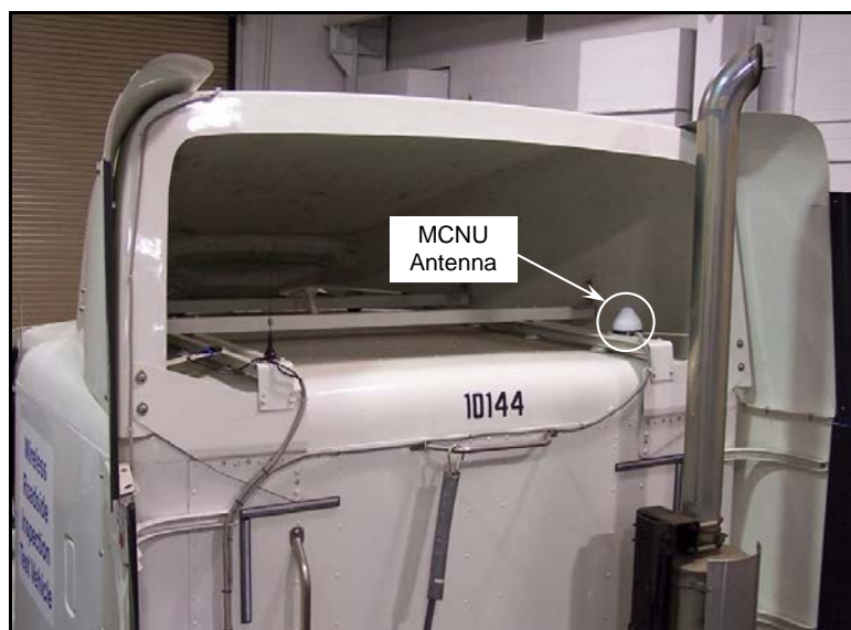
Figure 23. Photo. Placement of the MCNU Dome Antenna on WRI Test Truck
