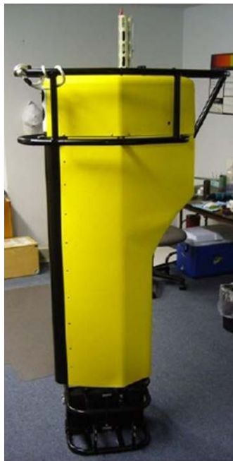
Figure 3-2. WET Labs AMP C100 In-Situ Profiler
