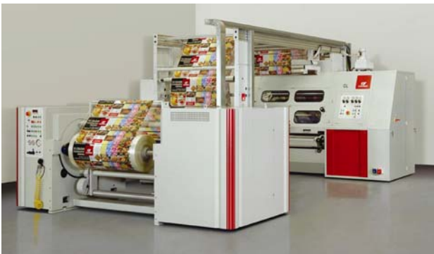
Biobased adhesives for flexible packaging have been processed on a commercial scale coater (pictured) at speeds of 1,000 feet per minute.
