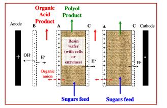
The separative bioreactor stack shows two cell pairs (cell is composed of membrane-resin-membrane stack). A commercial system could include up to 100 cell pairs.
