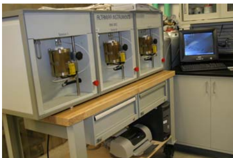
NREL's bench-scale catalyst microactivity test system.
