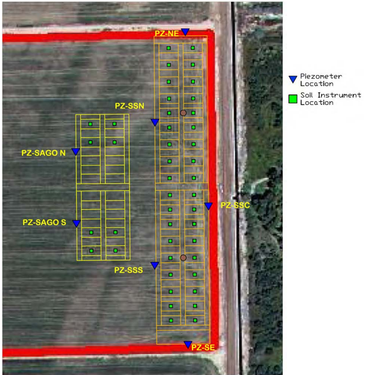
Figure 31. Instrumented well point piezometers and soil moisture monitoring locations in the small-scale study area.
