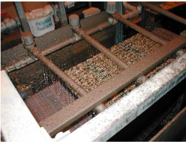
Figure 1. Tray/Cell Preparation —Automated cell preparation for cuttings. Soil and amendments such as fertilizers and vermiculite were inserted into each cell automatically.
