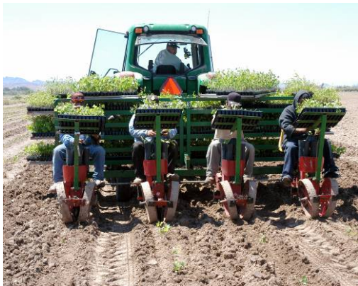
Figure 6. Field Preparation —Field was prepared for planting. A tomato planter filled with cottonwood and willow trees was connected to the tractor for planting.
