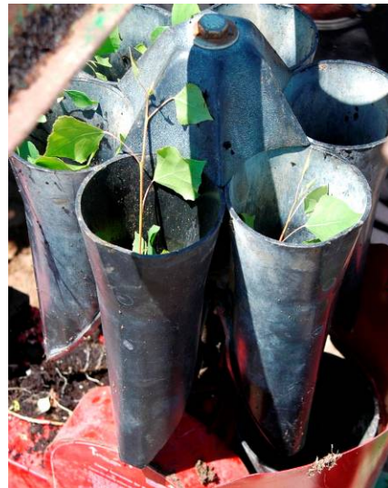
Figure 7. Feeder Funnels —Funnel feeder filled with cottonwood and willow trees. Trees dropped through at a designated rate for spacing of the trees.
