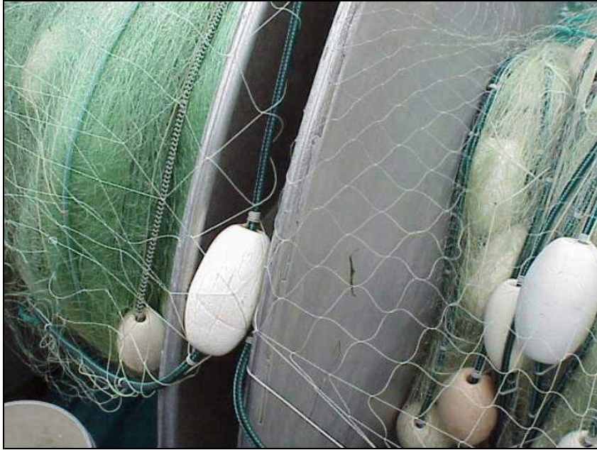
Figure 1. Photograph that shows conventional gill net (left) beside a tangle net (right). Photo provided by the Oregon Department of Fish and Wildlife Lower Columbia Management Office.
