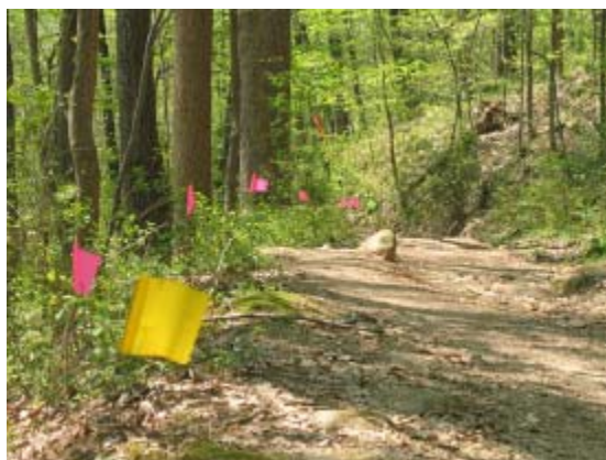
Figure 4. Left: Use of the measuring wheel to measure course. Right: Track marked with different colors of surveyor's tape. Yellow marked start, pink clearly marks track, green marks 25 meters.
