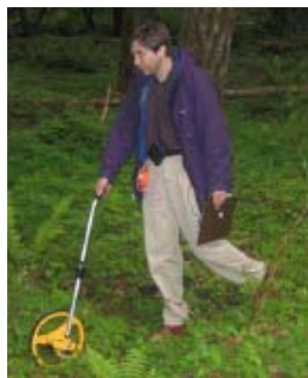
Figure 4. Left: Use of the measuring wheel to measure course. Right: Track marked with different colors of surveyor's tape. Yellow marked start, pink clearly marks track, green marks 25 meters.
