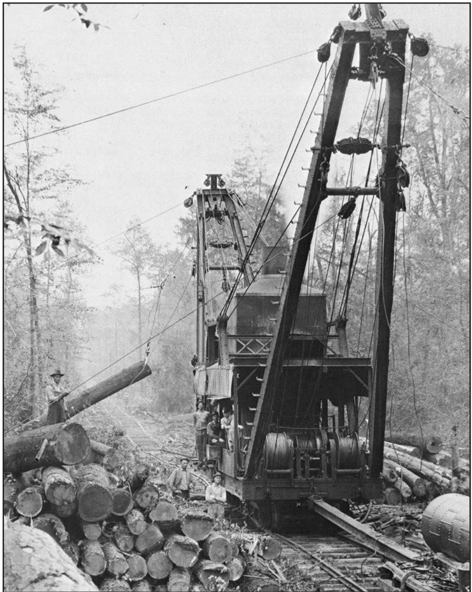
Clyde steam-powered skidders provided an efficient means of harvesting timber. However, they were extremely destructive knocking down any trees that were not cut.
