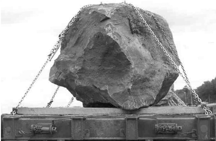
Chain is used to secure large boulders
