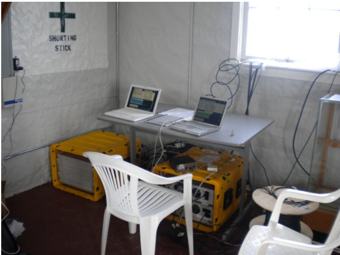
SeaSonde electronics and processing laptops side by side for both frequencies
