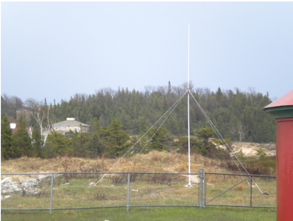
Long Range 5 MHz SeaSonde Transmit Antenna
