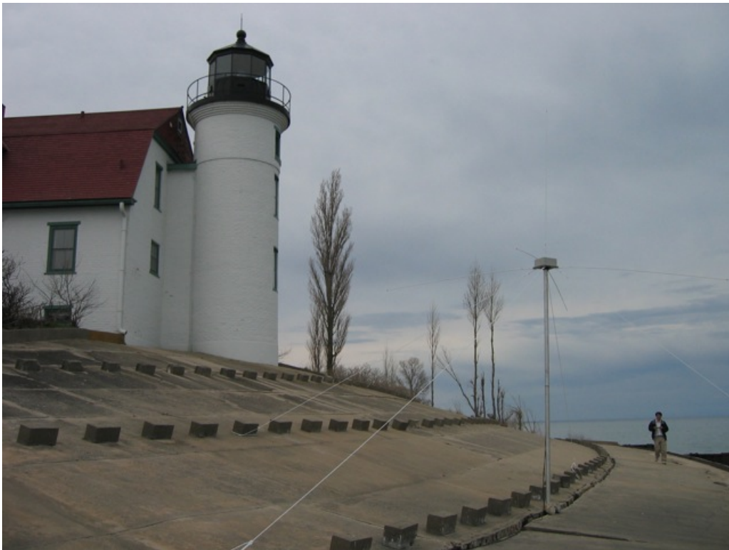
SeaSonde 5 MHz receive antenna in front of Pt Betsie Lighthouse
