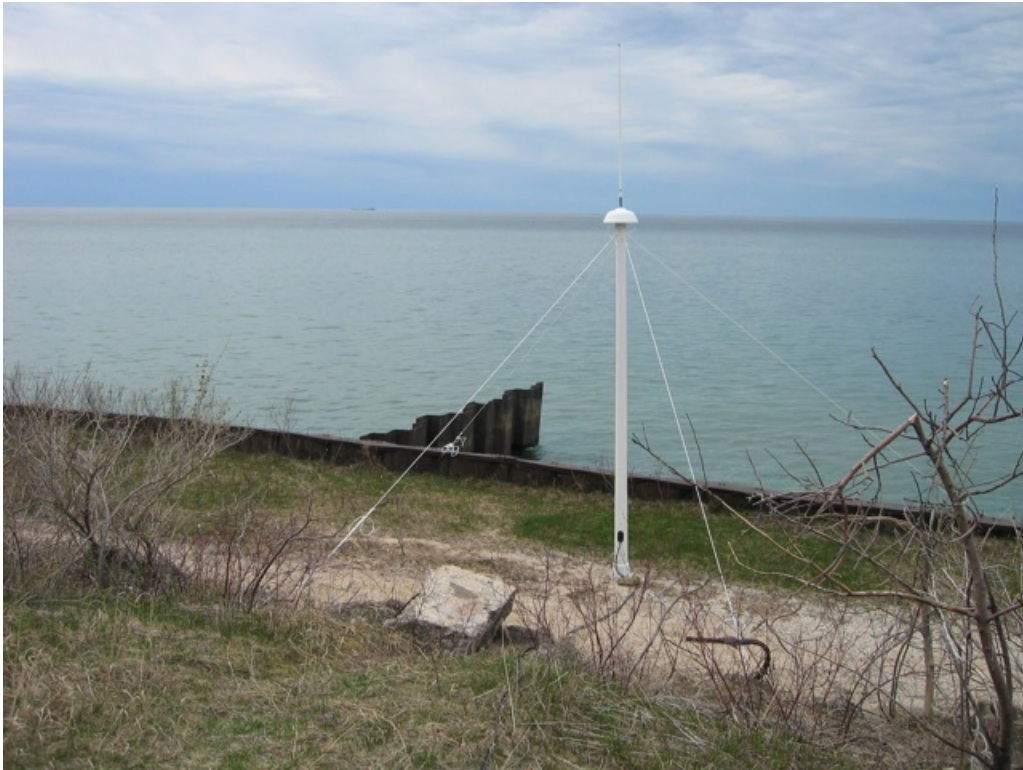
42 MHz SeaSonde Transmit/Receive Mast
