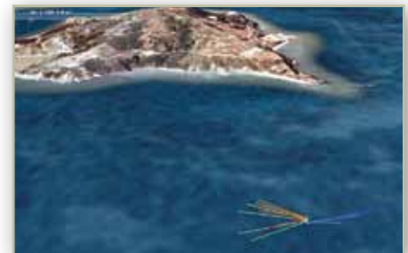
Snapshot of currents in Raccoon Strait, San Francisco Bay, CA, as sampled by two Acoustic Doppler Current Profilers. Red arrows are near the surface and blue arrows are towards the bottom. This snapshot was taken during the flood tide. The information is useful for boaters, sediment transport, and constraining an ocean circulation model for the San Francisco Bay. (Google)
