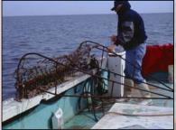
We used a modified crab scrape made of cold-rolled steel stock to dredge for terrapins in Chesapeake Bay. The scrape bar was 1.7 m wide and equipped with 30 15 cm downward facing teeth to help remove terrapins from bottom sediments. The scrape trailed an 8 cm-mesh knotted nylon bag to retain terrapins. Entrance to the bag measured 1.7m x 0.4 m.
