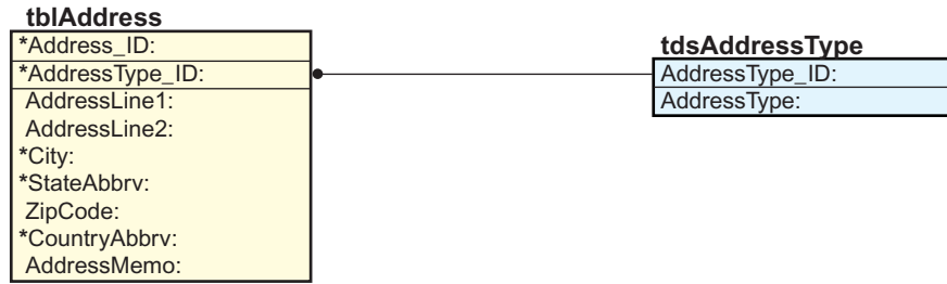
Figure 21. Address subject area tables, fields, and relationships. (Box represents a field coming from data tables, an asterisk represents a required field in data tables, and a black ball indicates a foreign key. See figure 18 for explanation of box color.)
