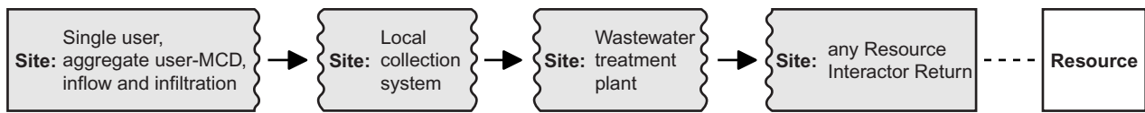
Figure 8. Return Network models 4, 5, and 6. (Dotted line represents a Site-Resource association, solid line represents a conveyance, and an arrowhead shows the direction of water movement.)
