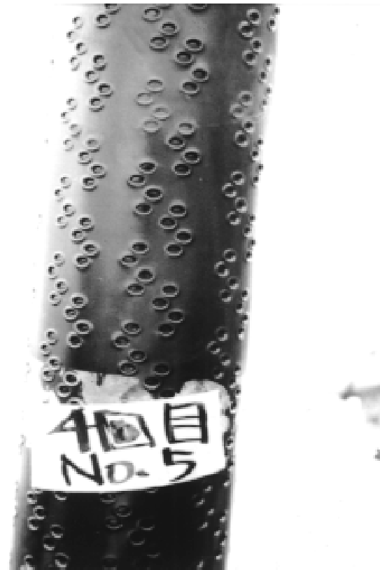
Figure 23. Dimple pipe used on stay cables on the Tatara Bridge.
