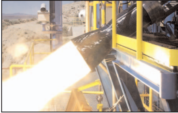
Low-cost, ablative composite rocket engine
