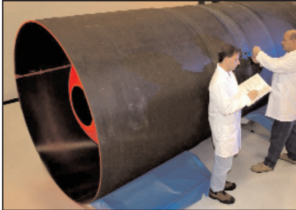
Subscale Composite Cryogenic Tank
