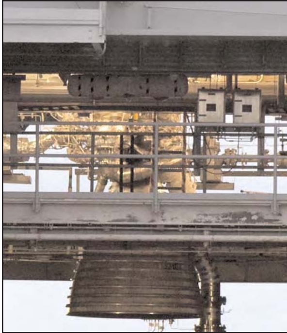
J-2 Awaits Testing on the A-1 Test Stand
