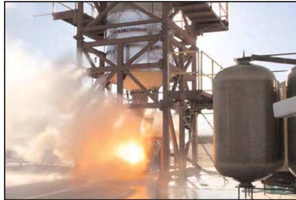
AirLaunch Hot Fire Test on VTS
