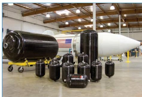
Family of all-composite propellant and pressure tanks
