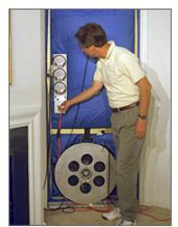
Blower door tests are often used in energy audits to determine the airtightness of a residence. Source: Department of Energy
