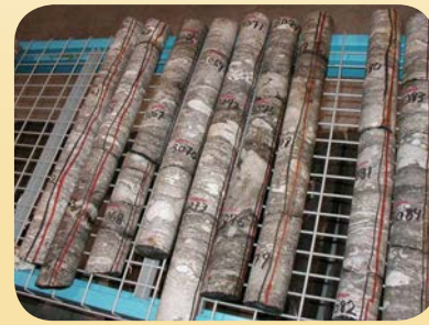
MRCSP rock samples collected and tested to assess their CO 2 storage resource potential.
