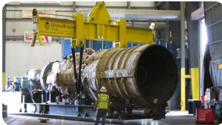
A turbine departs Siemens' facility for Clean Energy Systems' Kimberlina Power Plant in California, where oxy-combustion technology is being scaled up.
