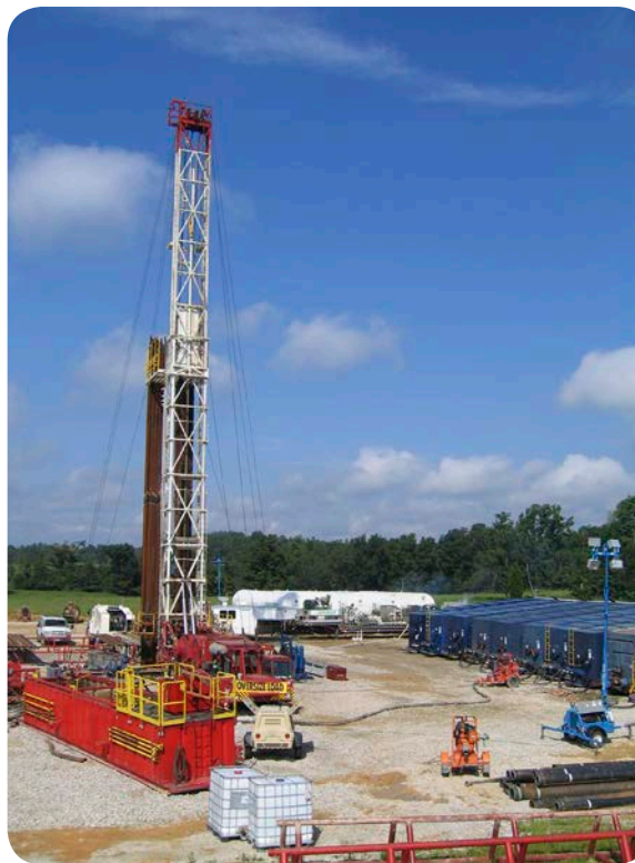
CO 2 injection testing in the Blan #1 well, Hancock County, Kentucky.
