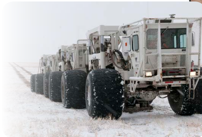
Seismic trucks used to generate 4-D data of subsurface.
