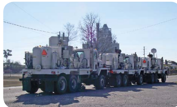
The 2-D seismic reflection acquisition by Bay Geophysical was collected using three Vibroseis trucks. The picture was taken along line SCO2-5.
