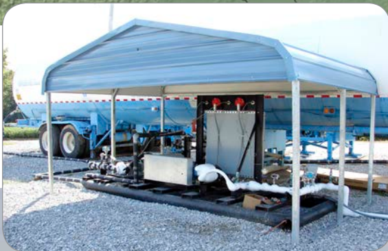
At left, Injection pump skid with CO 2 supply tanker in the background, Mumford Hills field EOR II site, Indiana.
