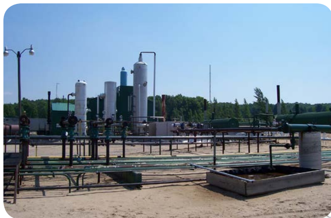
CO 2 separation and purification equipment at MRCSP large-scale field project site.
