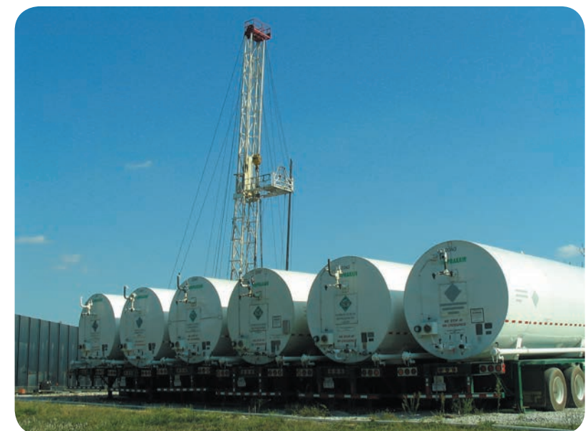
CO 2 storage tanks (Phase 2 injection) on the well site at the KGS' Marvin Blan #1 well, Hancock County, Kentucky.
