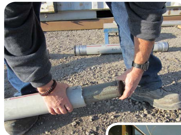
Pulling whole core from the core barrel.
