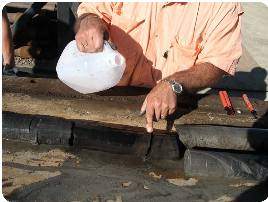
Field inspection of freshly collected lignite core.
