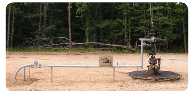
CO 2 -EOR production wellhead. (Photo courtesy of TX BEG)
