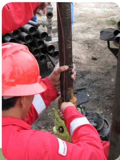
Installation of downhole pressure sensor.
