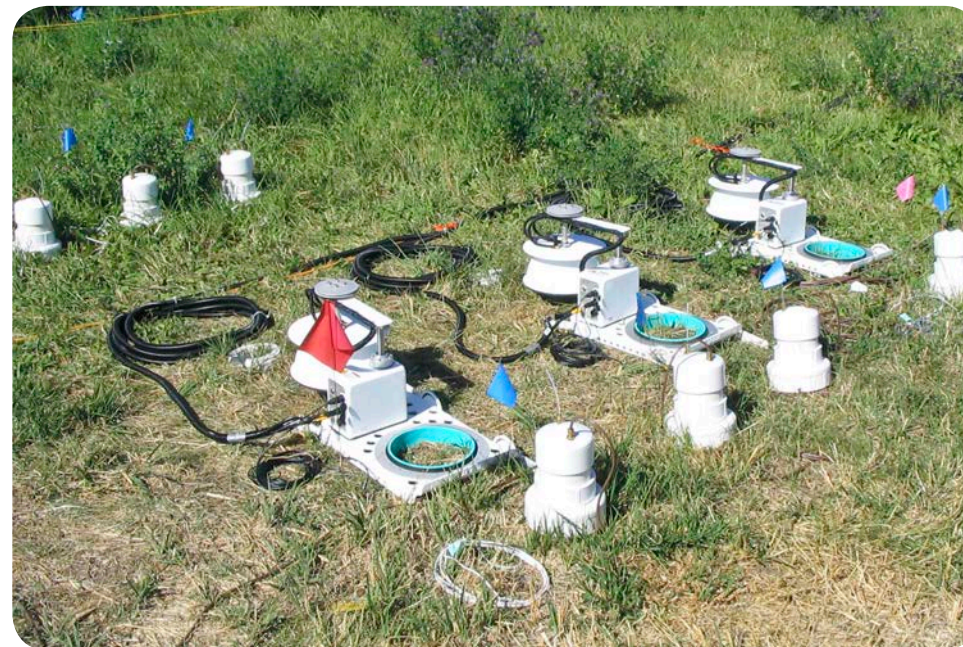
Soil gas chambers analyze CO 2 levels in the soil. (Photo courtesy of Jennifer Lewicki)
