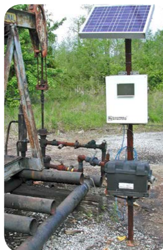
Reservoir monitoring well at the Sugar Creek field EOR III site, Kentucky.
