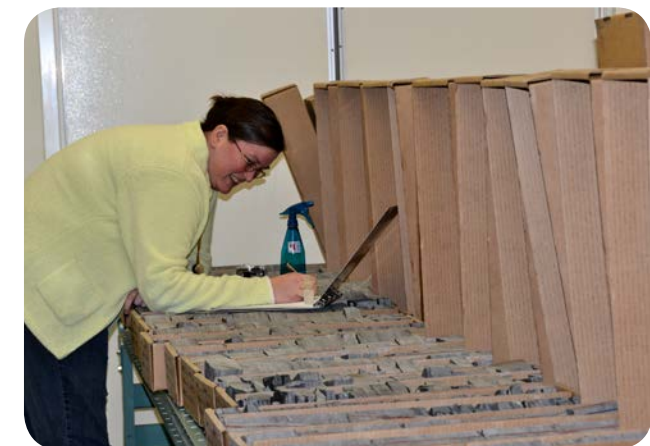
Geologist describing core of a sealing shale formation that was recovered from the Gorgas #1 borehole.
