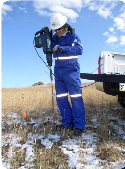
Driving a probe to collect a baseline soil gas sample in the Bell Creek oil field.
