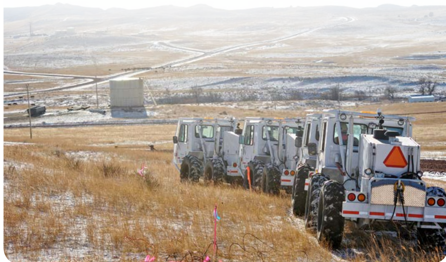
Mini vibe trucks conducting a check shot survey as part of a seismic source testing exercise in the Bell Creek oil field.
