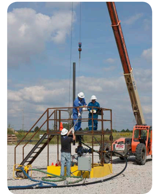
Fluid sampler being retrieved from the IBDP verification well.
