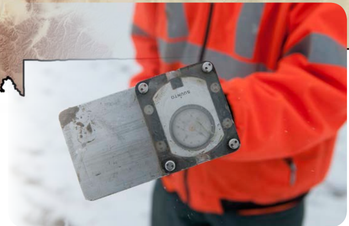
Instrumentation used to align seismic components in the field.
