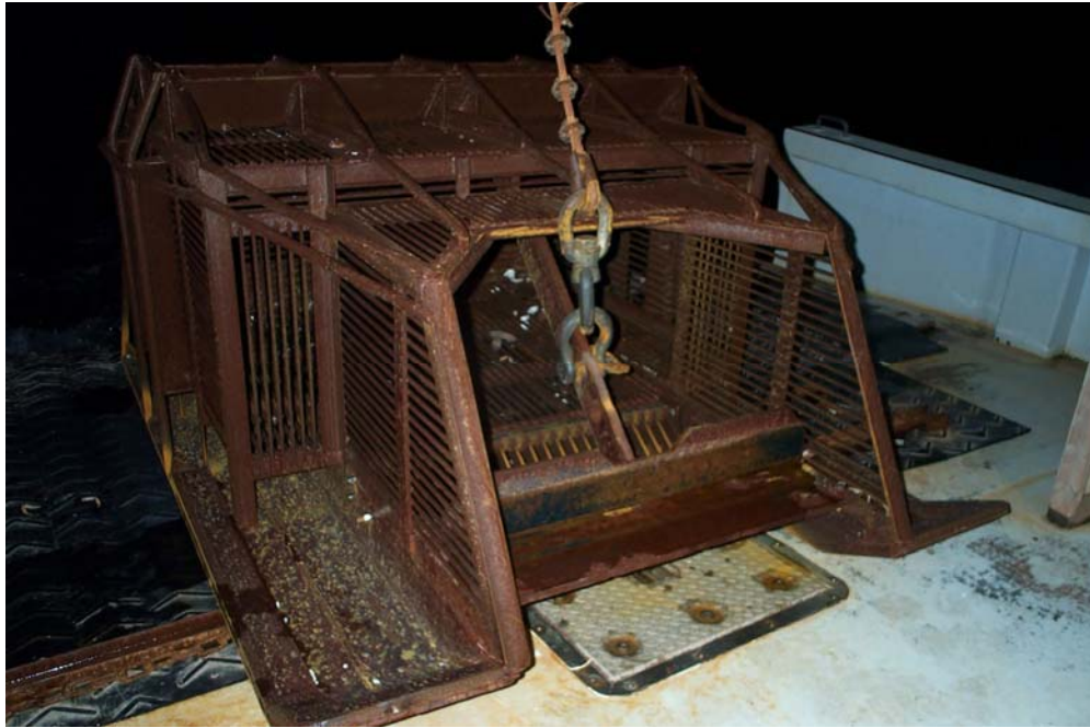
Appendix A8. Figure 5. Commercial drag used in all surveys in 2005.
