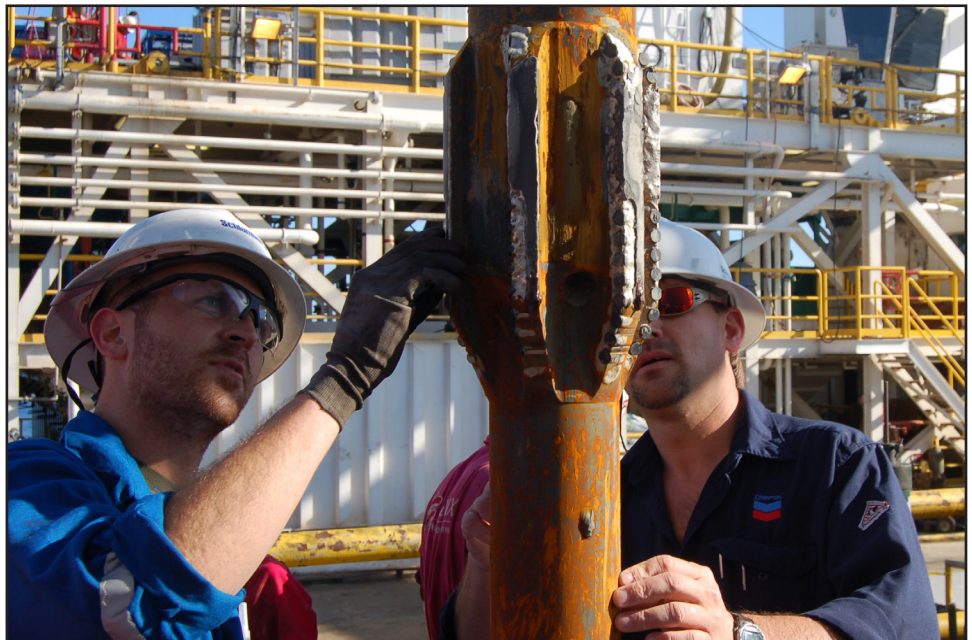
• Figure 1: Schlumberger and Chevron personnel inspect drillstring onboard the Q4000, the floating drilling unit used on Leg II.
