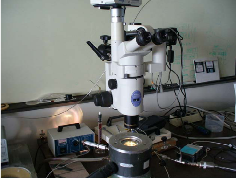
Cell for study hydrates in porous media. P=300 bar
