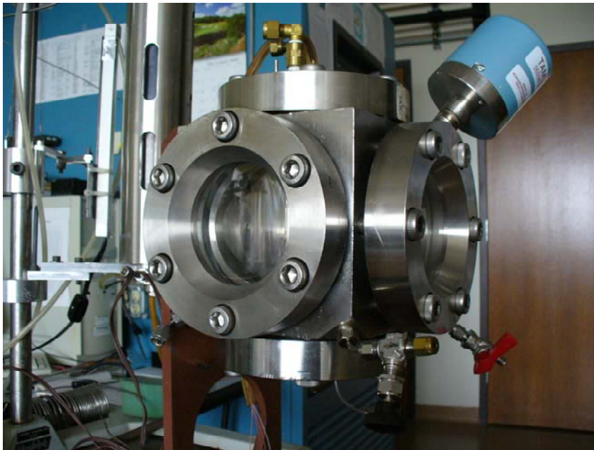
Cell for study hydrates in porous media. P=300 bar
