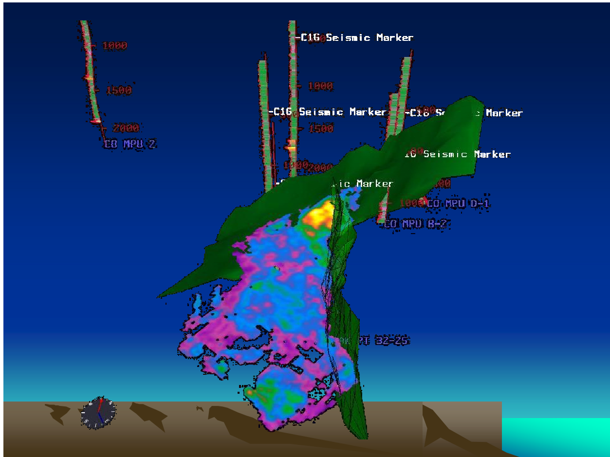
Figure 22: Three dimensional display of the Mt. Elbert prospect with the bounding faults and adjacent key wells.
