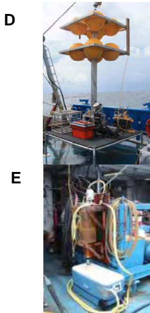
Figure 2. Principal equipment used during HYFLUX cruise. A. RV BROOKS McCALL, B. Global Explorer ROV with niskin sampler array. C. Rosette. D. Elevator with instruments and sampling equipment. E. Seawater equilibrator for surface sampling. F. Science party
