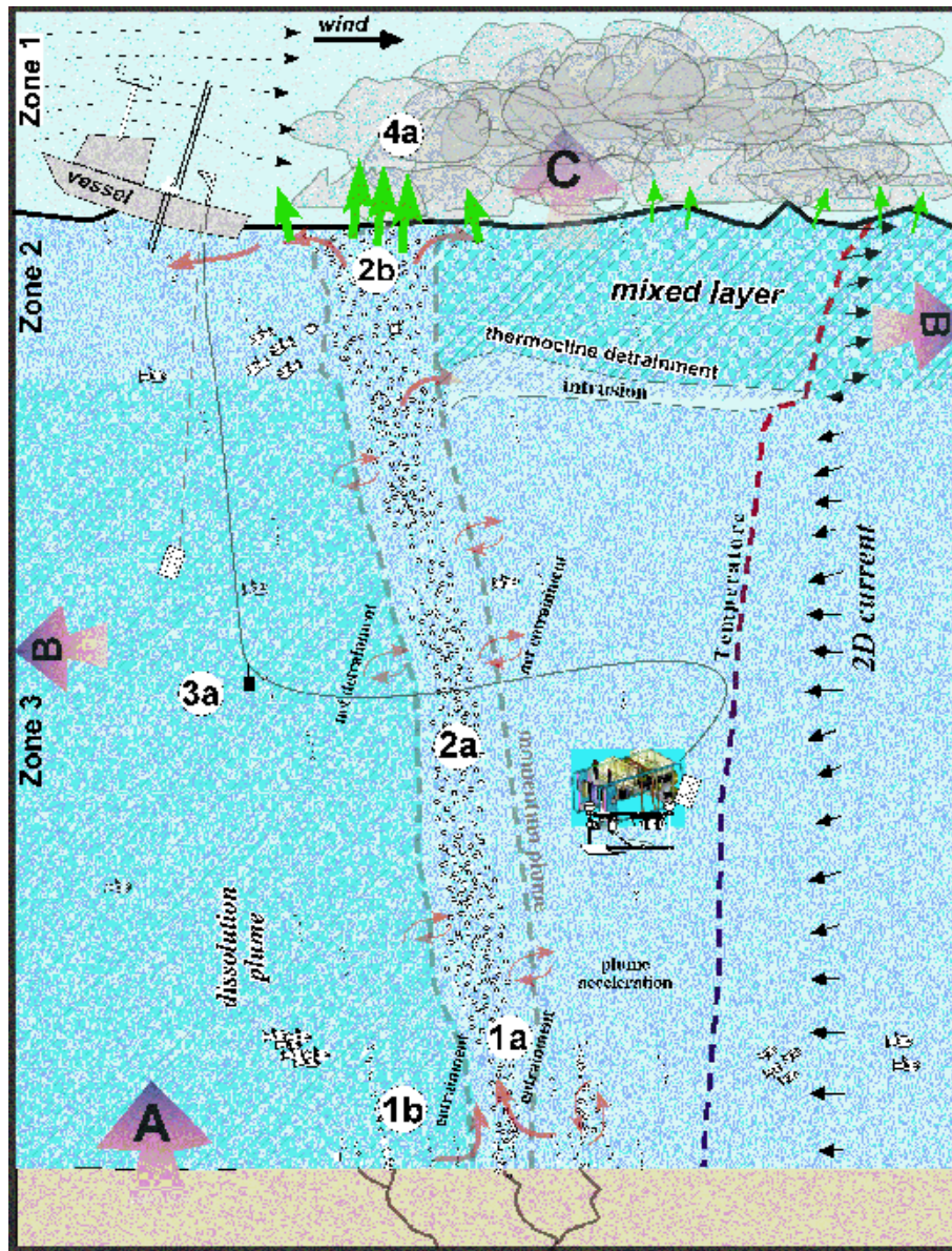
Figure 3.1: Schematic showing bubble plume processes.
